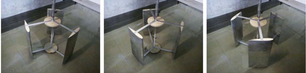
**Fig. 6: Mock-up blade tests at low flow velocities ( $v \approx 0.4$  m/s)**
